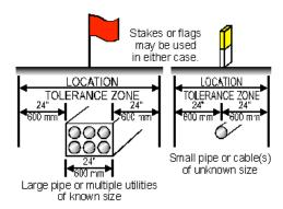
To avoid damaging underground facilities an excavator shall determine the precise location of underground facilities which have been marked. Accepted industry opinion is that precise determination can only be made by exposing the buried utility. Depending on site conditions, one, or a combination of the following options, is recommended: careful hand digging
