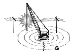
Instruct all other personnel to stay at least 30 feet away from the equipment, ropes, and the load. The entire equipment, load, and the ground around it could be energized.
